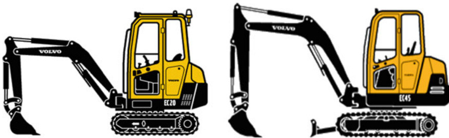
Fig. 1 The two models of mechanical shovel used: (EC20) a 2-ton mechanical shovel with a three cylinder engine; (EC45) a 4.5-ton mechanical shovel with a four cylinder engine
