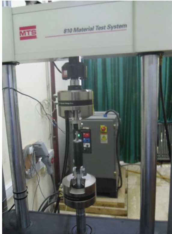
Fig. 2 Characterization of the MR damper (RD-1005-3) on fatigue machine 'MTS 810'
