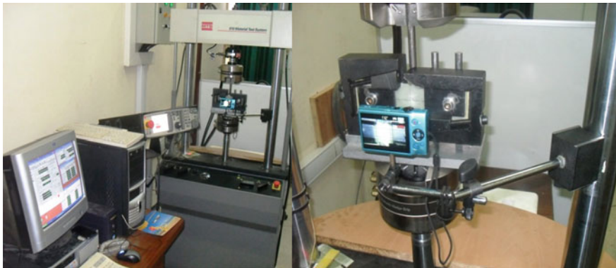
Fig. 4 Iosipescu device mounted on a MTS 810 machine
